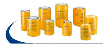
Filter element Spin-On, working pressure 12/35 bar (174/508 psi), flow rates up to 250 l/min (66 gpm), threaded connections 3/4" BSP 1" - 12 UNF 1 1/4" BSP 1 1/2" - 16 UN
