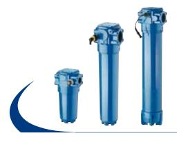
In-line filter, working pressure 50/60 bar (725/870 psi), flow rates up to 740 l/min (195 gpm), threaded connections from 1 1/2" and 2" BSP/NPT/SAE and flanged connections 2" and 2 1/2" SAE 3000 PSI.
