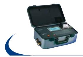
Particle counter calibrated to ISO 11171 standard, working pressure from 2 bar (29 psi) to 400 bar (5801 psi). Contamination reports data in ISO 4406, NAS 1638 and AS4059 formats. Oil temperature and relative humidity reading sensors.
