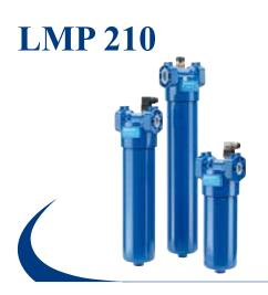
In-line filter, working pressure 60 bar (870 psi), flow rates up to 300 l/min (80 gpm), threaded connections from 1" to 1 1/2" BSP/NPT/SAE and flanged connections up to 1 1/2" SAE 3000 PSI.
