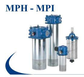
Tank mounted return filter with oil flow internal to external filtering element. Working pressure 10 bar (145 psi), flow rates up to 2000 l/min (530 gpm), threaded connections from 1/2" to 1 1/2" BSP/NPT/SAE and flanged connections SAE 3000 PSI/DIN up to 4".
