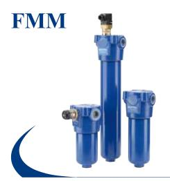
In-line filter, working pressure 420 bar (6091 psi), flow rates up to 150 l/min (40 gpm), threaded connections up to 3/4" BSP/NPT/SAE/ISO 6179.
