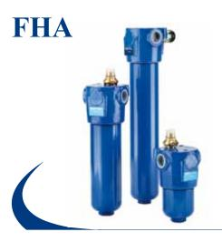
In-line filter, working pressure 520 bar (7540 psi), flow rates up to 150 l/min (40 gpm), threaded connections up to 3/4" BSP/NPT/SAE/ISO 6179.
