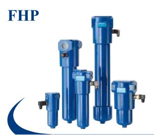
In-line filter, working pressure 420 bar (6091 psi), flow rates up to 475 l/min (126 gpm), threaded connections up to 1 1/2" BSP/NPT/SAE and flanged connections up to 1 1/4" SAE 6000 PSI.
