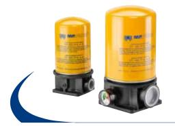
Tank mounted return filter Spin-On, working pressure 12 bar (174 psi), flow rates up to 200 l/min (53 gpm), threaded connections from 3/4" and 1 1/2" BSP/NPT/SAE and flanged connections 1 1/2" SAE 3000 PSI.
