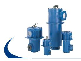
External suction filter, flow rates up to 550 l/min (145 gpm), threaded connections up to 1/2" to 2 1/2" BSP/NPT and flanged connections up to 3 1/2" SAE 3000 PSI.
