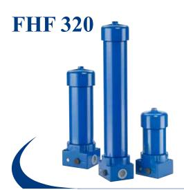
In-line filter, working pressure 350 bar (5076 psi), flow rates up to 500 l/min (133 gpm), threaded connections 1 1/2" BSP/NPT/SAE and flanged connections 2" SAE 6000 PSI manifold type.
