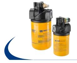
In-line filter Spin-On, working pressure 35 bar (508 psi), flow rates up to 250 l/min (66 gpm), threaded connections from 3/4" to 1 1/2" BSP/NPT/SAE.
