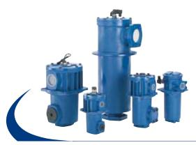
In line or tank mounted return filter with oil flow external to internal filtering element. Working pressure 20 bar (290 psi), flow rates up to 1500 l/min (397 gpm), threaded connections from 1/2" to 2 1/2" BSP/NPT/SAE and flanged connections up to 3 1/2" SAE 3000 PSI.
