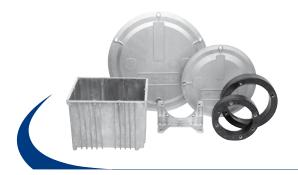
10-litre aluminium tank, inspection doors of diameter 350 and 475 mm conforming with DIN 24339 and feet for mounting bell-housings on B3 motors with power range from 0.25 to 22 Kw.
