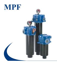
Tank mounted return filter, with oil flow external to internal filtering element. Working pressure 8 bar (116 psi), flow rates up to 750 l/min (198 gpm), threaded connections from 1/2" to 2" BSP/NPT/SAE and flanged connections up to 2" SAE 3000 PSI.
