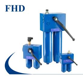
In line duplex filter, working pressure 350 bar (5076 psi), flow rates up to 345 l/min (92 gpm), threaded connections from 1/2" to 1 1/4" BSP/NPT/SAE and flanged connections 1 1/2" SAE 6000 PSI.
