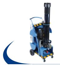
UMF 090 – 180 mobile filtration units suitable for filling and refilling of filtered hydraulic fluids and lubrication tanks. Flow rate 90/180 l/min. Pressure max. 10 bar. Electrical motor: 3 phase UFM 918 two-speed electric motor with programmable flow of 90 or 180 l/min. Pressure max. 10 or 6 bar. Electrical motor: 3 phase
