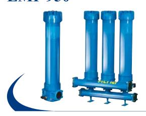
In-line filter, working pressure 30 bar (435 psi), flow rates up to 2000 l/min (528 gpm), flanged connections 3" and 4" SAE 3000 PSI.
