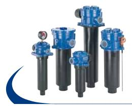
Tank mounted return filter with oil flow external to internal filtering element.
