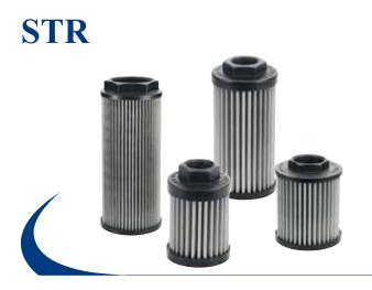
Submerged suction filter, flow rates up to 900 l/min (238 gpm), threaded connections from 1/2" to 3" BSP/NPT.
