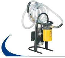
The GRF 015 is a portable oil transfer/filtration unit, specifically designed for both filling/transferring hydraulic oils from containers to the hydraulic tank as well as filtering and cleaning hydraulic systems. Flow rate 15 l/min. Pressure max. 5 bar. Electrical motor: single phase.
