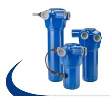
In-line filter "Suction/Return", working pressure 80 bar (1160 psi), flow rates up to 160 l/min (42 gpm), threaded connections 1" BSP/NPT.
