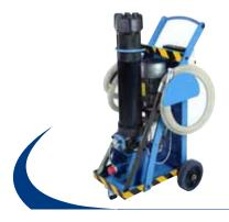
UMF 040 mobile filtration units suitable for filling and refilling of filtered hydraulic fluids and lubrication tanks. Flow rate 33 l/min. Pressure max. 5 bar. Electrical motor: single and 3 phase.
